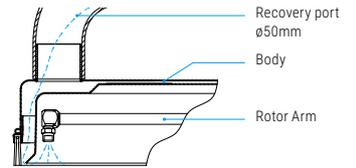
Residual water and debris can be recovered, recycled and reused.
