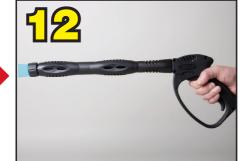
Open the trigger gun and the pump will slowly start to prime the water through
