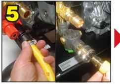
Attach the water suction hose to the machine inlet connection
