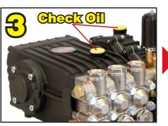
Check the oil levels for the pump, and gearbox (if fitted)
