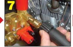
Attach the high pressure hose to the machine outlet connection
