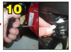
Open the fuel tap, close the choke and start the engine, gradually open the choke until the engine runs smoothly
