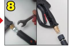
Attach the end of the high pressure hose to the trigger gun connection
