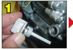
Fill engine with oil to correct level
