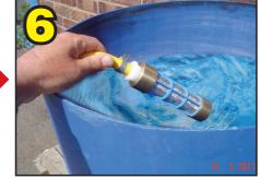
The suction hose should be used with a clean water supply
