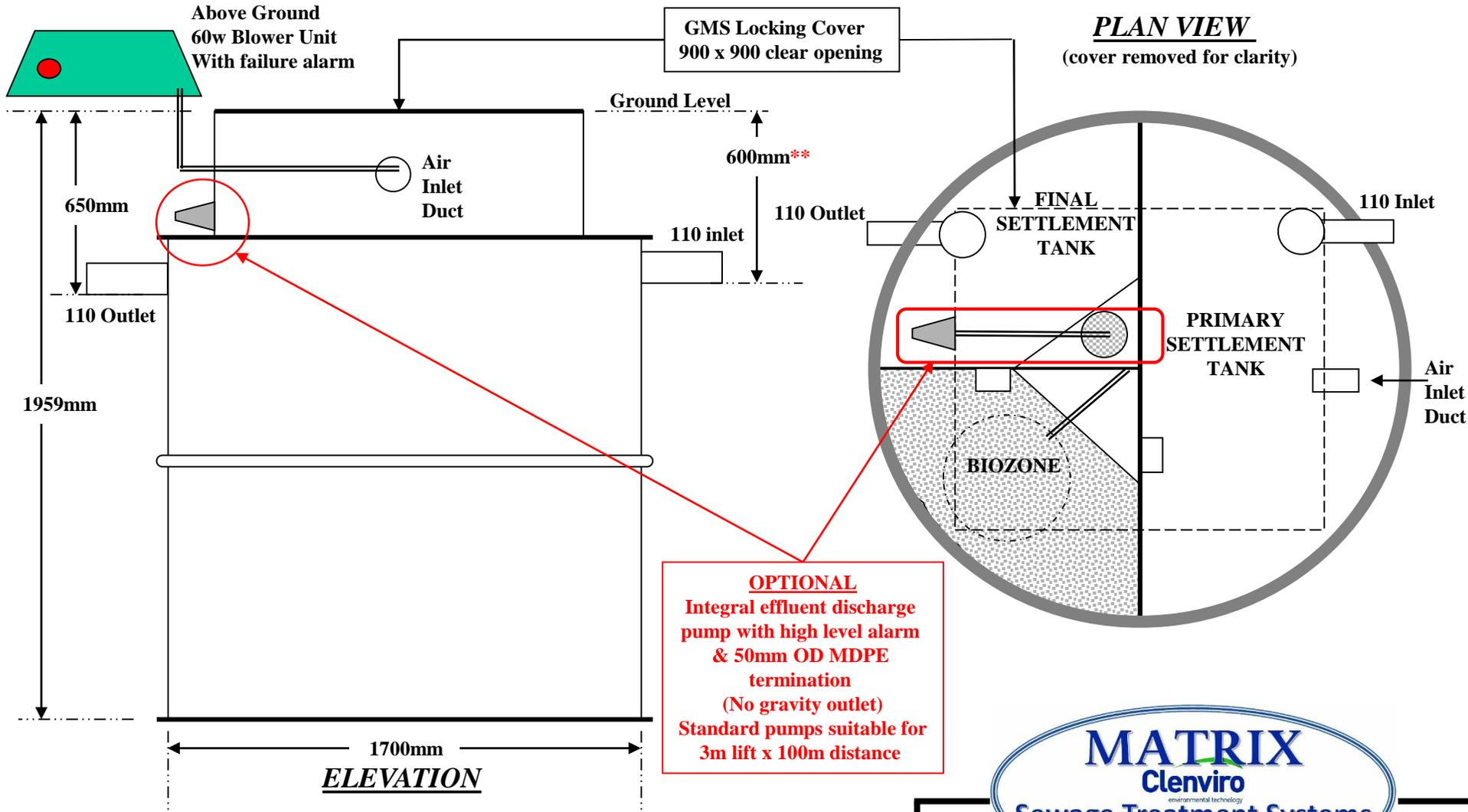
**\*\* Alternative inlet inverts can be accommodated at time of order/manufacture. Retro-fit (after delivery of the tank) access extensions in excess of 500mm height will invalidate any structural warranty.**
