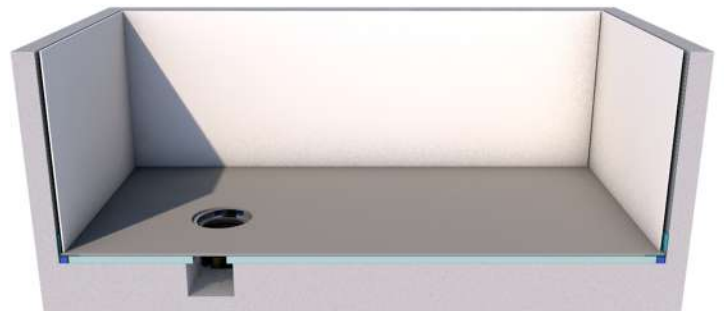
4. Concrete base is poured, wall batons and dry wall applied.
