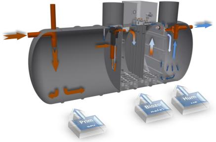
The system utilises micro-organisms to break down the sewage by processes very similar to those that occur in a garden compost heap. It is very important therefore, that toxic chemicals do not enter the system and "poison" the micro-organisms.
