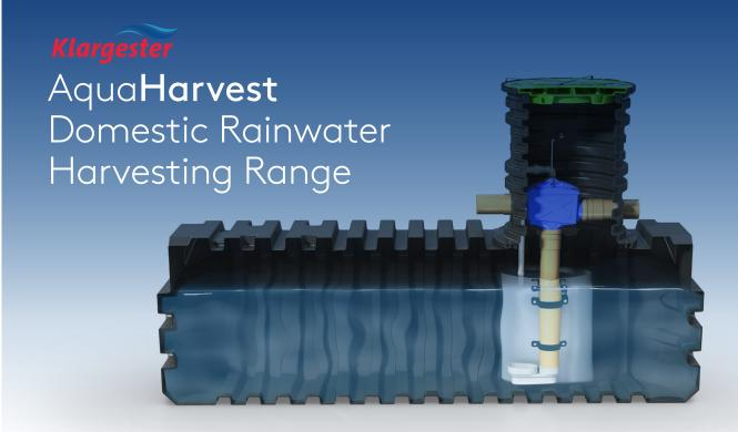
The AquaHarvest rainwater solution is a Direct System suitable for domestic applications. This system is used where it is impractical to have a header tank, for example in homes that have converted attic spaces and less room. Therefore, filtered rainwater is pumped direct from the holding tank to the various appliances.
