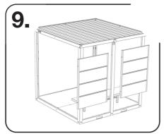
Lift each wall panel into place between upright and middle support then secure in place using M8 fixings. Ensure the ribs/ pressings of the side panels face inwards. Now re-check every single fixing on the Forma-Shelta and ensure no fastener is loose.
