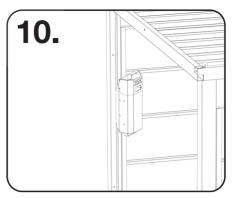
The cigarette bin can slot into any upright without fixings. To remove, lift upwards and out.
