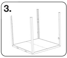
Tighten the two front uprights using a 19mm socket but leave the rear uprights hand tight.
