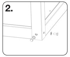
Attach uprights to each corner of the base using 2x M12x25mm bolts with washers.
