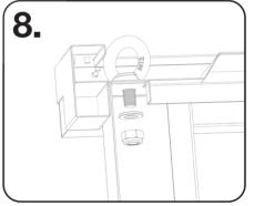
Insert an M12 crane lifting eye from the top in each corner of the roof and through the slot in the top of the upright below. Secure lifting eyes with M12 washers and Nylock nuts.
