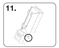
Before disposing of waste, ensure no embers are left burning. Pull the plunger on the rear of the lid to open and empty into a general waste bin. Close lid and reattach to the Forma-Shelta.
