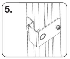
Slot the lugs of the folding bench into the brackets and tighten rear uprights to base.
