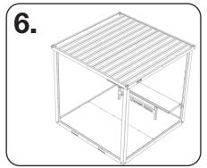
The roof can now be lifted onto the uprights and located by the channels running under the roof in each corner.
