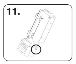
Before disposing of waste, ensure no embers are left burning. Pull the plunger on the rear of the lid to open and empty into a general waste bin. Close lid and reattach to the Forma-Shelta.
