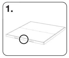
To begin assembling the Forma-Shelta, place base on a level, stable surface. The front of the unit can be configured from any side but we recommend the forklift pockets are at the front.
