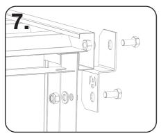
Next the middle supports for side panels need to be fitted, one on the back and each side. Slide the top of the support under the roof first and then fix to the base using M12x25mm bolts and washers. The top can then be fixed using the supplied bracket and M12 fixings as shown.
