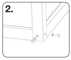
Attach uprights to each corner of the base using 2x M12x25mm bolts with washers.
