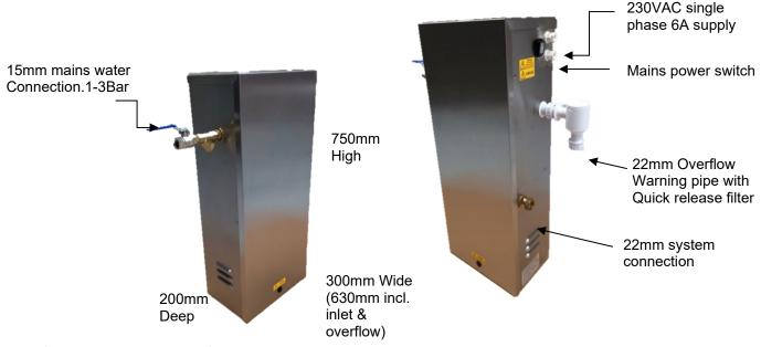
Fig. 1.2 External Connections
