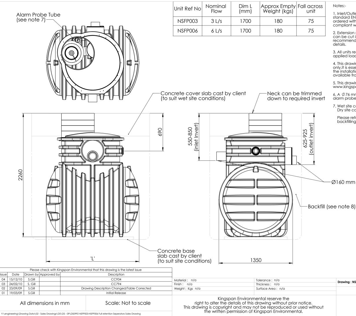
1. Inlet/Outlet pipes are plain pipe  $\emptyset$  160 mm PVCu. The standard EN 858 states minimum connection sizes, units ordered with different sized connections are not fully compliant with the standard.
