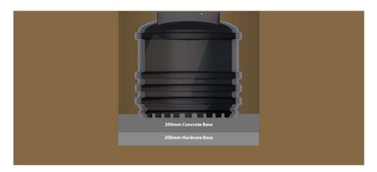
17.3. Fill chamber with a minimum of 700mm water in readiness for the first concrete pour.
