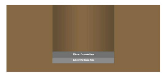
17.2. Place chamber in the center of the excavation and position firmly into the damp concrete base. Ensure the chamber is level and in the correct position.
