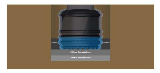
17.6. Repeat the process for the second pour, once again ensure that the water level exceeds that of the concrete. Ensure vibration takes place at each stage of the concrete pour.
