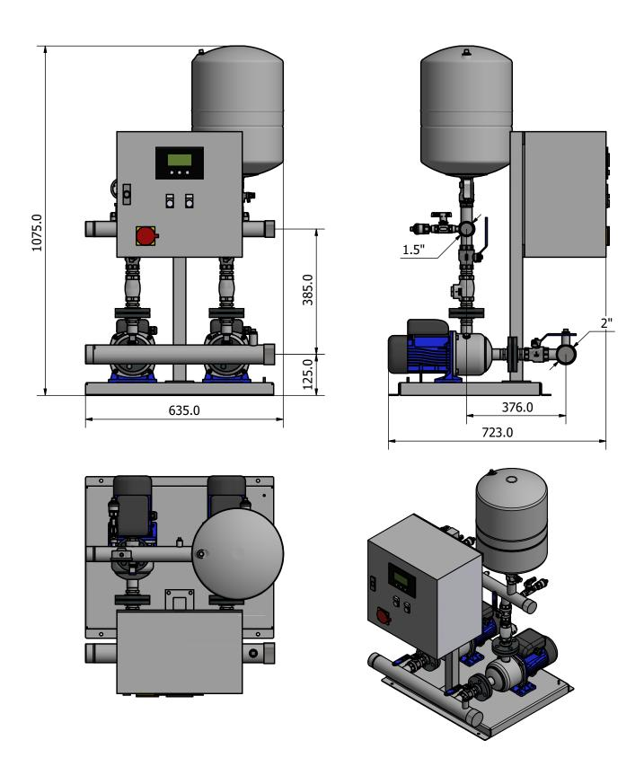
\*Please add 32mm to the total height from the base of the pump when AV mounts are used.
