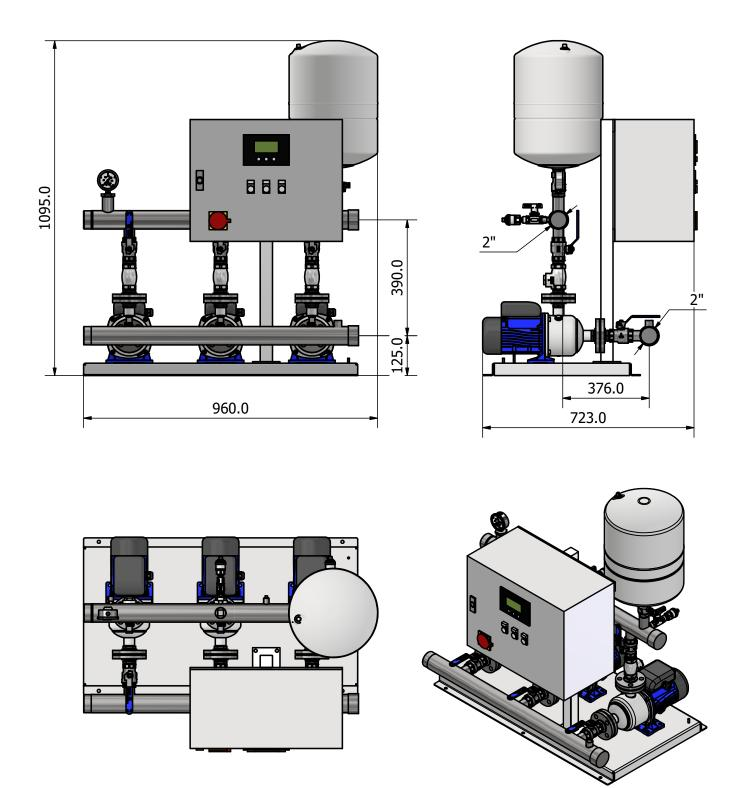
\*Please add 32mm to the total height from the base of the pump when AV mounts are used.
