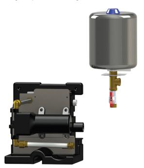
Mount the 3/4" flexible hose on the connection of the pressure side of the pump (bottom connection). Then, mount the other side of the flexible hose at the bottom side of the mounting bracket. Use the fiber rigns for a water tight seal.
