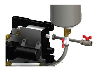
Connect the 3/4" F connection on the T-piece under the pressure tank on the secundary water network. Once all the pipings are connected water proof, you can continue commissioning.
