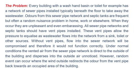
**The Solution:** Install a Poly-Air activated carbon vent filter to prevent the odour problem by removing the offensive odours such as Hydrogen Sulphide as they exit the sewer network vent pipes.
