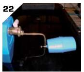
The plastic float valve height can be adjusted to set the water level in the trough.
