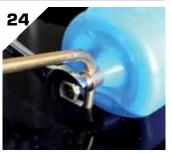
Select the desired water level and tighten the bolt on the slider to secure the float position.
