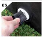
Using the plug key provided unscrew the plug and allow the water to drain.
