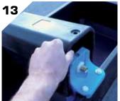
Position the ballcock cover over the ballcock support.
