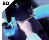
Engage the thread of the float valve inlet & elbow fitting and rotate the float valve assembly to tighten.
