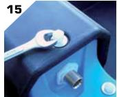
Place a nylon screw and a s.steel washer through the hole on top of the ballcock cover into the threaded hole on the ballcock support below. Then tighten.
