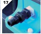
Place the assembly on the end of the float valve inlet. Align the threads correctly then tighten.
