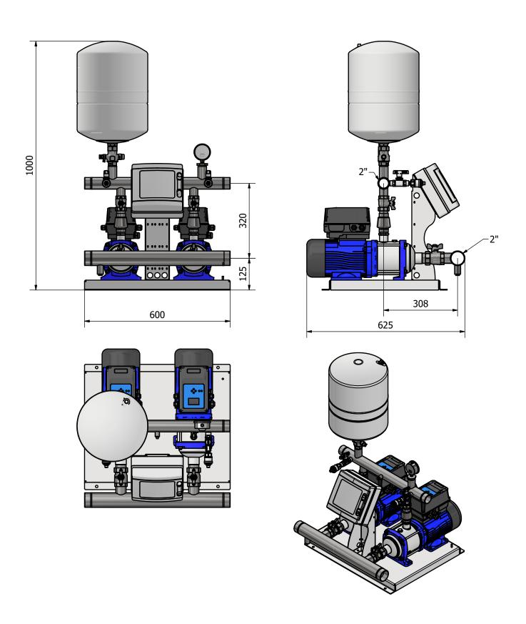
\*Please add 32mm to the total height from the base of the pump when AV mounts are used.
