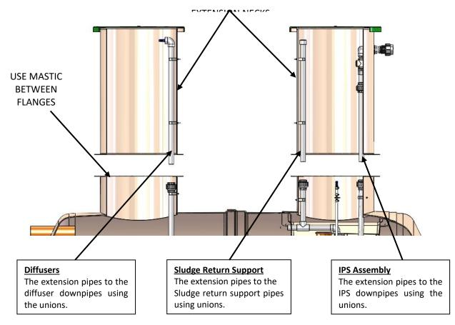
When the installation includes a separate structural concrete raft, it is necessary to order the extension kit to the full invert depth. The full invert depth is from finished ground level, Failure to take account of the finished ground level will mean that the internal valves and junction boxes will not be accessible for routine maintenance and servicing. This may require "confined space" entry which will significantly increase the cost of maintenance and servicing.
