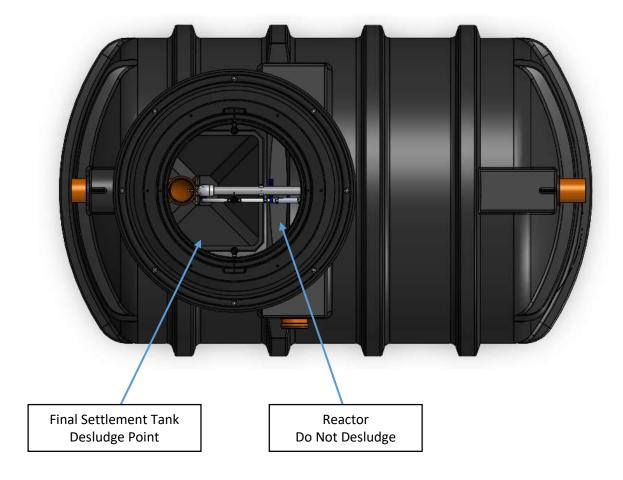
Insert the suction hose into the FST, taking care not to damage the sludge return pipework. Approximately 300mm of active sludge must remain in the bottom of the reactor.
