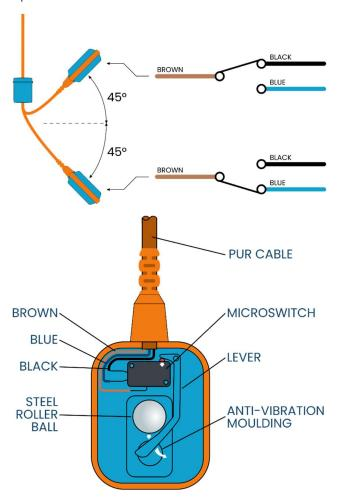
**NOTE:** The float switch must be securely tethered or fitted with a counterweight to ensure correct operation
