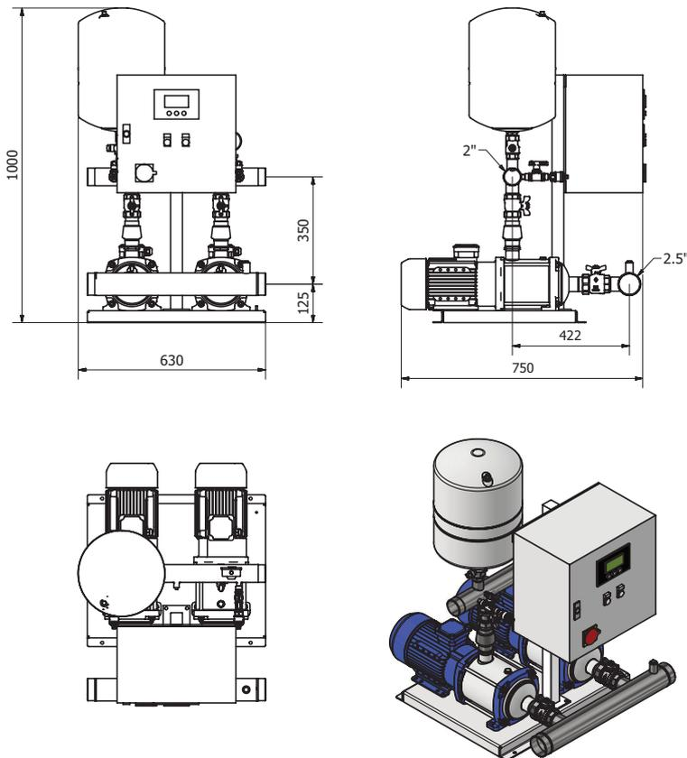
Please add 32 mm to the total height from the base of the pump when AV mounts are used.
