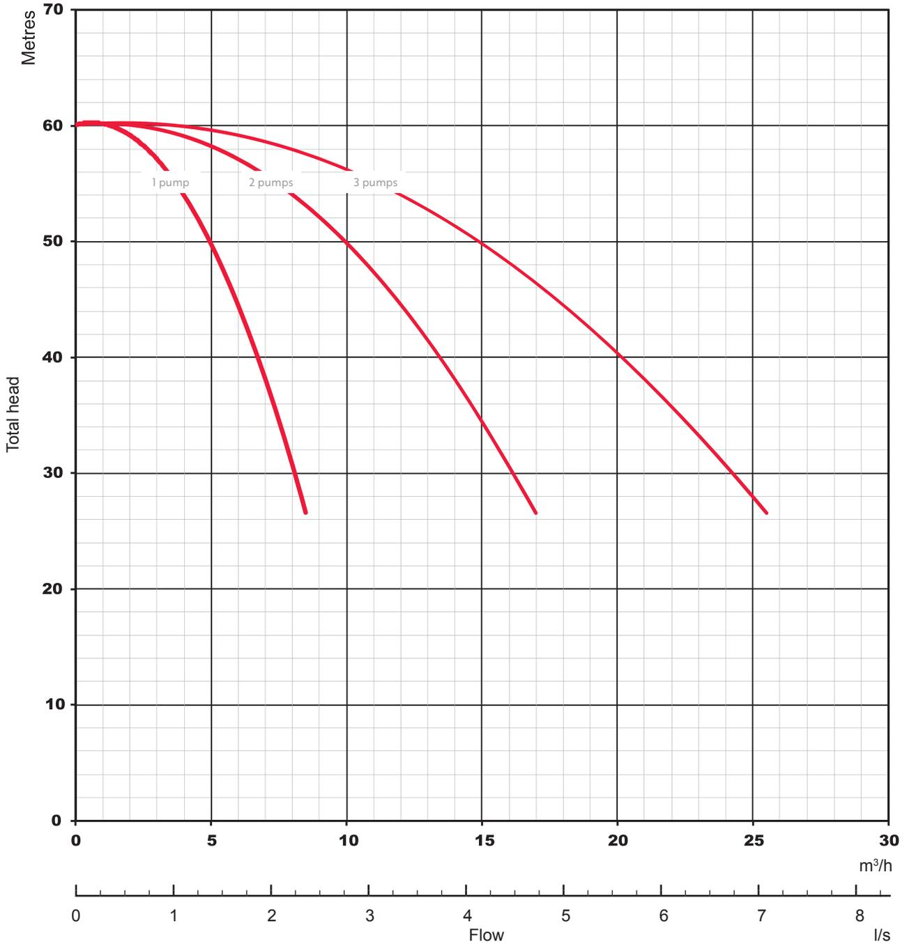
Performance curve is in accordance with ISO 9906:2012 Grade 3B Tolerances.
