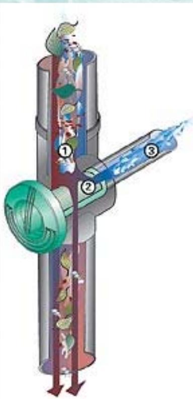
1. Rainwater is channelled from the filter entrance to the sieve cartridge.
