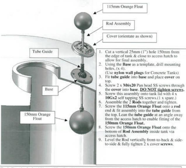
Tools Required: 2 x 150mm (6") adjustable spanners, 25mm ø (1") Hole saw or drill, 3.5ø (1/8") Drill Bit, 8.0ø (5/16" & 1" Masonry drills - concrete only), # 2 Philips screw driver & spirit level.
