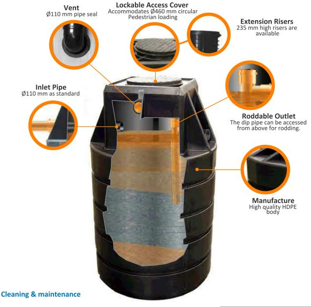
The GS range of separators are designed for containment and NOT treatment. Secondary products and dosing systems are available introducing chemicals/enzymes that can break down the accumulated Fats, Oils and Grease.
