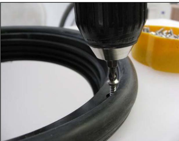
Place neck ring in tank, Using 6 stainless self tapping screws, screw neck ring into tank. Screw location marked by dimples in the neck ring.
