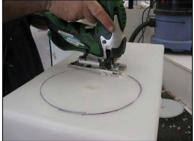
Using a jigsaw cut around the line to make a hole.
