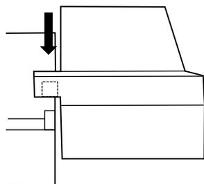
Fill both sides to pocket underside
