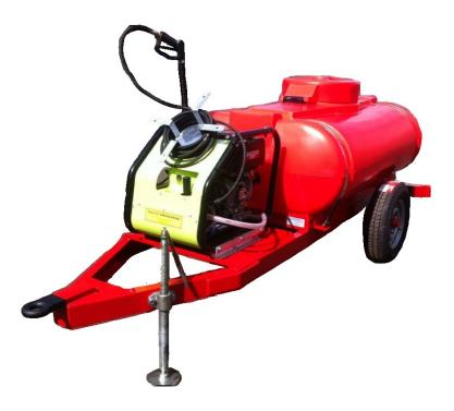
**CHASSIS:** Constructed from 100 x 50 RSC fully welded, with front standing plate and an 'A' frame drawbar, 80x80x6 RSA frame, hot dipped galvanised.
