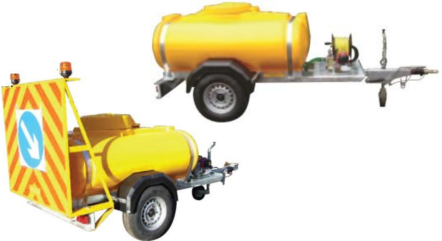
**CHASSIS:** Constructed from 80 x 80 RSA. fully welded with a 'T' frame drawbar, all fully hot dipped galvanised. 5mm sheet front mounting plate.
