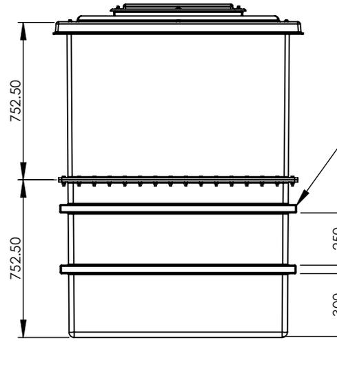
2 No 40mm Encapsulated RHS Steel Bracings
