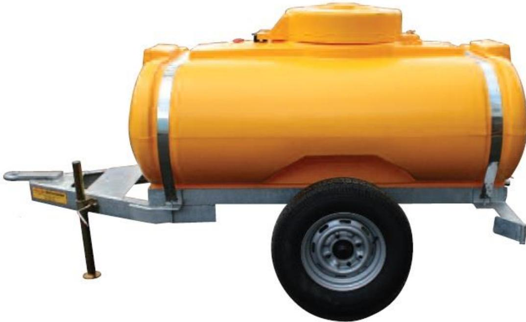
**CHASSIS:** Constructed from 100 x 50 RSC fully welded, with front standing plate and an 'A' frame drawbar, 80x80x6 RSA frame, hot dipped galvanised.
