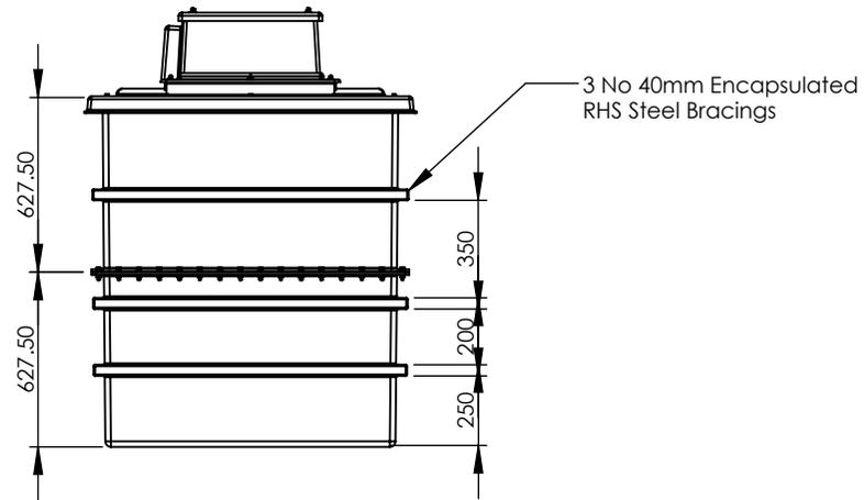
3 No 40mm Encapsulated RHS Steel Bracings
