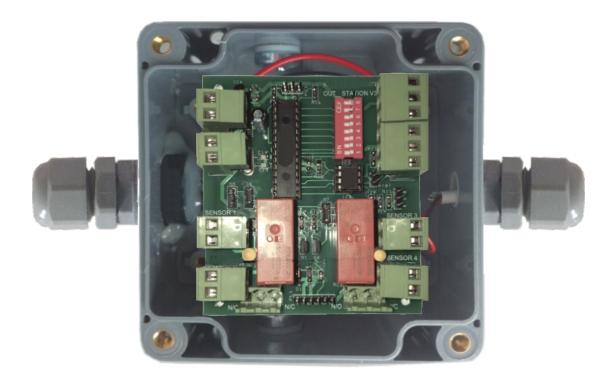
A maximum of 100 four zone outstations can be connected to one LeakMonitor alarm panel giving a multizone system capable of monitoring 400 different areas simultaneously.
