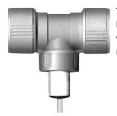
The tee sensor has been designed to go into the over flow pipes on break tanks, toilet cistern and header tanks. The sensor is located inside the tee piece and gets installed on the overflow pipe with the sensor at the bottom. Any water that travels down the pipe and into the tee sensor will make contact with the conductors of the sensor and set off the alarm.
