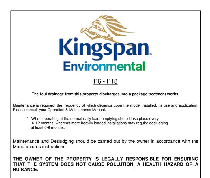
We recommend that a separate log is kept of all maintenance and service visits, the log should detail the date and any action taken, e.g. Regular maintenance service, breakdown visit, desludge volume removed, parts replaced.
