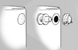
with rubber bung supplied. Push Rainsaver connector through the washer from the inside, then fit and tighten the nut on the outside to form a seal.
