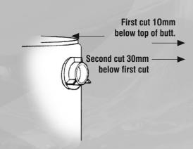
It will be helpful to release any clips supporting the downpipe, in order to insert the Rainsaver body, but these should be re-fitted on completion.
