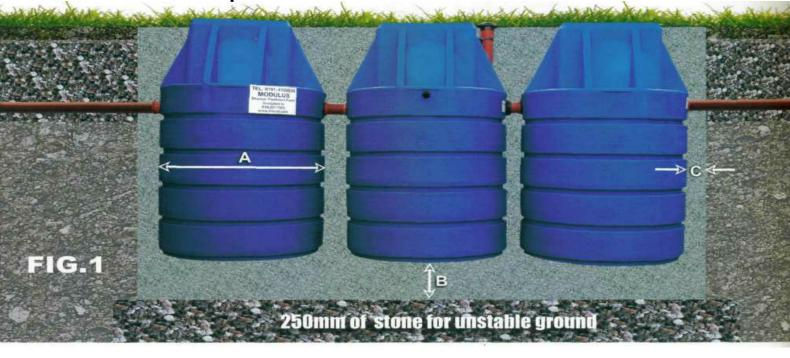
Illustrations below show standard installation in good ground using no formwork
